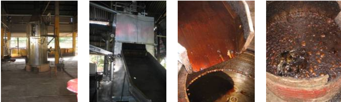
Picture 14 Steaming and roasting machinery, oil remains and oil outlet (from left to right)
